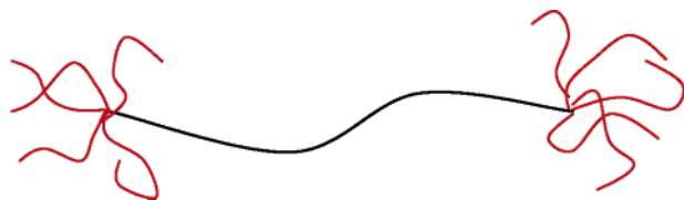
Scheme 1. Schematic of a Pom-Pom Molecule with 5 Branches (Red) Grafted at Each Backbone End.
